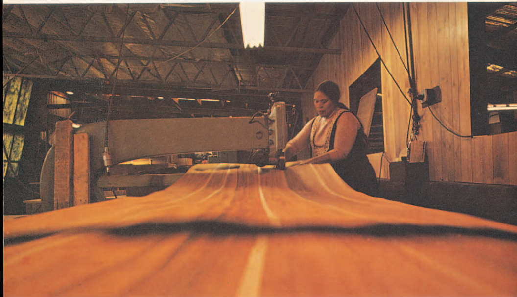
Matching and taping Rimu veneer. Scott Group is New Zealand's largest veneer dealer.
